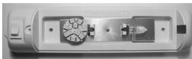
Comparison of standard 10 watt G4 halogen with a 2.2 watt plug in replacement LED
